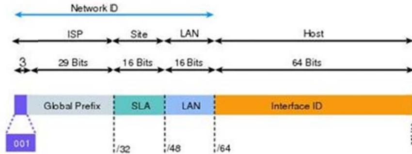
The host portion of the IPv6 address is called the Interface ID, because it does not identify the actual host, but rather the host's network interface card. Each network interface can have multiple IPv6 addresses, and therefore, can also have multiple interface IDs.
